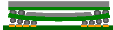
Figure 2 Open joints due to warpage
