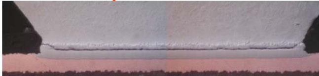
Figure 14: Drop test failure analysis of top package joints (ball + SOP)
