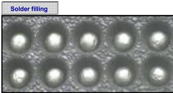
Figure 6: Solder balls in TMV openings
