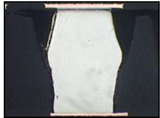
Figure 12: Cross section of PoP solder joint after attaching top package
