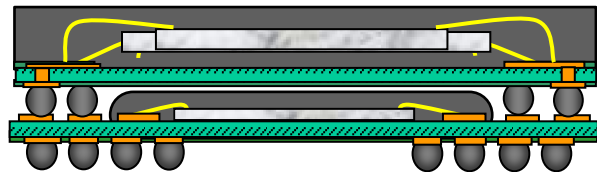
Structure 1. Bottom package - wire bond, center gate mold package structure: has warpage control, thickness, die size, dual or stacked die, passive integration and memory interface density limitations.
