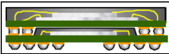
Figure 1: Standard Wirebond PoP configuration with exposed PoP land pads highlighted to stand out.
