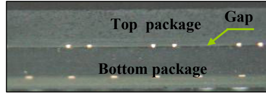
Figure 11: Gap between top & bottom package after pre stacking
