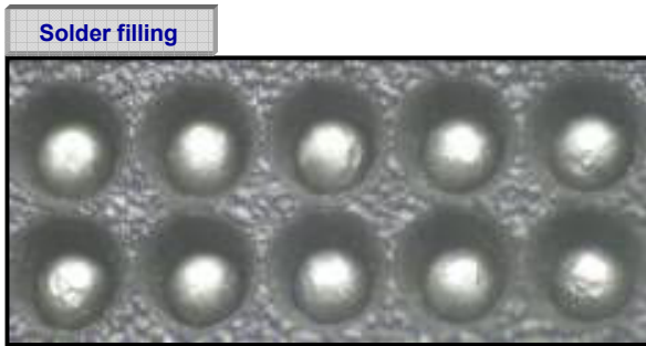
Figure 6: Solder balls in TMV openings
