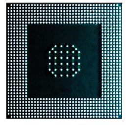
These components have a 1.0mm pitch with perimeter ball alignment and the tray quantity is 21. Minimum order quantities may apply.
